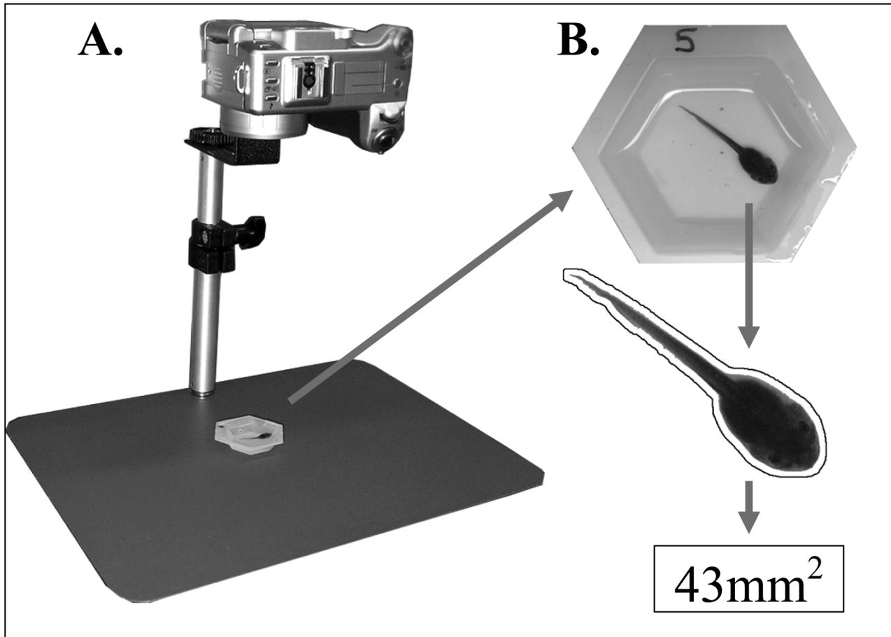
FIG. 1. Camera and photography stand used to photograph tadpoles in the lab and field (A). Tadpoles were held in white plastic weighing boats filled with water during photography. Later, digital images of tadpoles (B) were examined using Fovea Pro software. In the program, the entire tadpole was selected and its dorsal surface area measured in  $\text{mm}^2$  based on a previously defined pixel-to-mm ratio obtained from a ruler image.
