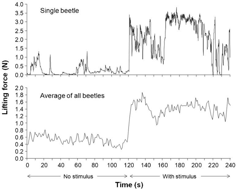
**Fig. 2** Lifting force measurements over time for one beetle (*top*) and for all 20 beetles in this experiment (*bottom*). Bottom graph shows average force readings of all beetles every second. Error bars not displayed for clarity. Note the difference in scale between both graphs. All trials lasted 4 min, and beetles were not manipulated during the first 2 min. For the last 2 min, the hind end was gently and continuously tapped with a blunt probe
