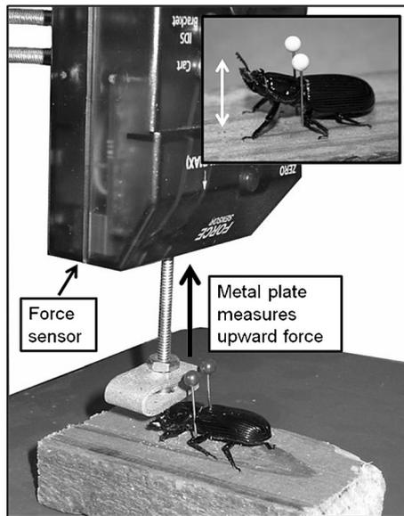
**Fig. 1** Measurement of beetle lifting force. Beetles were positioned on a wooden block using insect pins placed on either side (inset figure), and were positioned under a force sensor that recorded the continuous lifting force produced at the head and prothorax region (see Fig. 2 for force readings)
