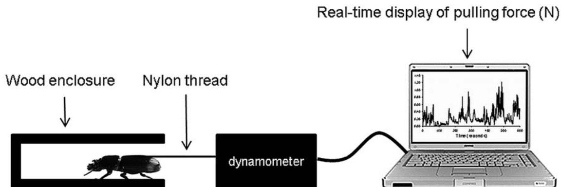
**Fig. 2.** Schematic of the apparatus used to measure pulling strength of *Odontotaenius disjunctus* in this study.
